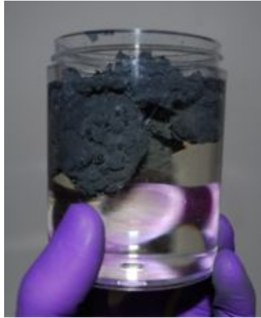
Figure 14: Gel slurry of nAl and n-pentane added to HTPB for further mixing.
