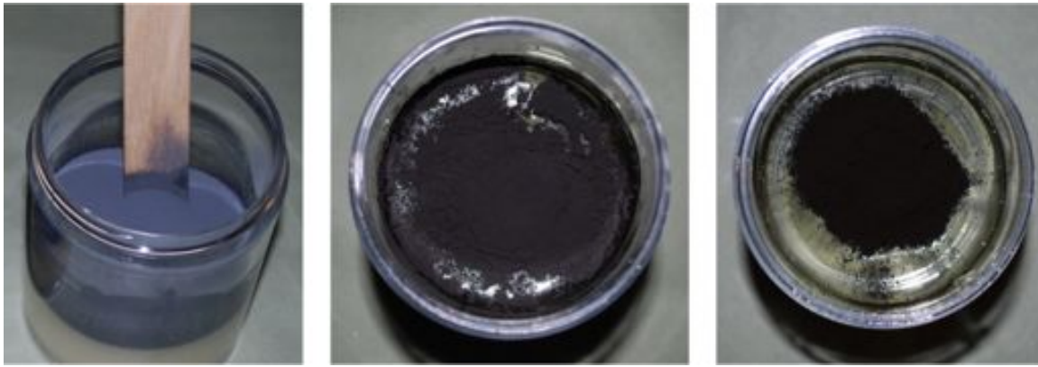
Figure 10: Initial weighing of nanoaluminum (left), nanoboron (center), and Copper Oxide nanorods (right) in HTPB.
