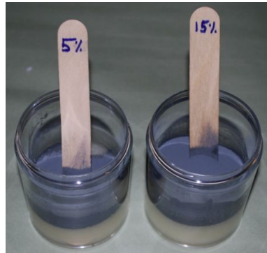
Figure 17: Preparation of 5% and 15% nAl samples in HTPB, pre-wetting, with 143L MDI added.
